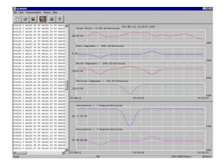
Separate charts are displayed to the right and are arranged in sequence with Total Field, East, North and Vertical components in a designated plotting area. Below are Inclination and Declination charts that provide easy visualization of changes in inclination and declination.
