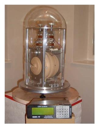
The Suspended dIdD comprises a revolutionary small diameter (250 mm), spherical Overhauser sensor with a bidirectional set of bias coils. Data is acquired directly to a GEM Overhauser magnetometer.
