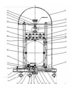
Even if the base or suspending part is tilted, the two springs ensure that the coil remains in the same position. This also applies to the tier or pedestal on which the system rests.
