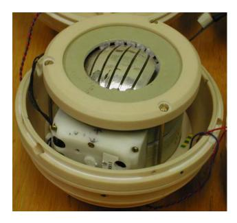
The external casing is impact resistant plastic. An upper support plate ensures that there is no movement of the sensor.
