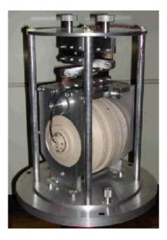
A simple algorithm is used to determine the instantaneous angular differences between the coil axes and the direction of the Earth's vector, **F**. These angular differences are dI and dD.
